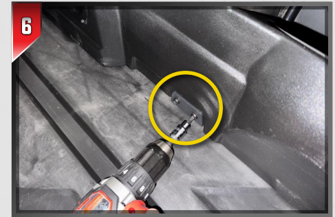
6 With the provided hardware, secure the middle mounting bracket to the subwoofer enclosure.
