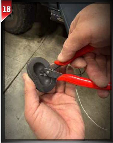
You will need to cut a small hole into the firewall plug to be able to pass the power wire through.
