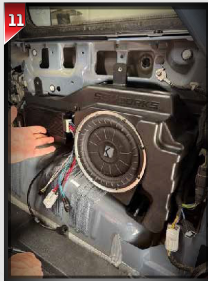
11 Reuse factory hardware to mount sub box into location using 10mm socket Tighten top bolts first then bottom bolts.
