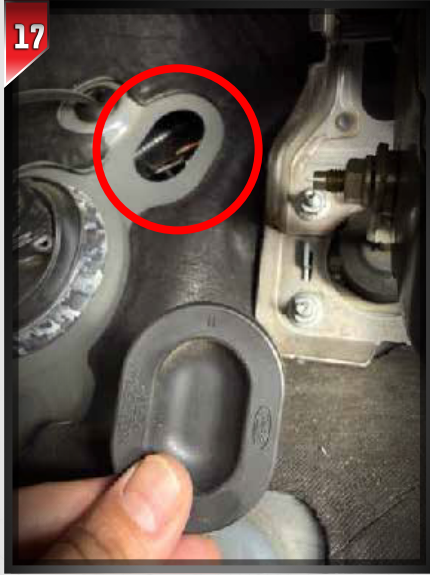
You can now remove the firewall rubber plug to able to run the power wire to the battery.
