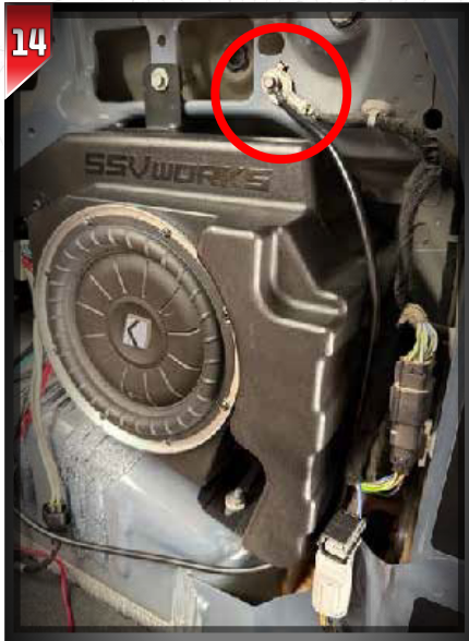
Disconnect the ground wire that runs above the subwoofer enclosure using an 8mm socket, then connect the subwoofer ground wire in the same location.
