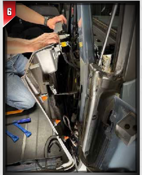
6 You can now fully remove the passenger panel to expose the factory subwoofer and connections.
