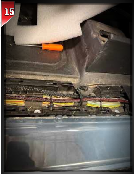
Using a panel popper, remove the bottom rear and driver side door trim pieces to expose the wiring to be able to run your power wire up to the front of the vehicle to make your connection to the battery.
