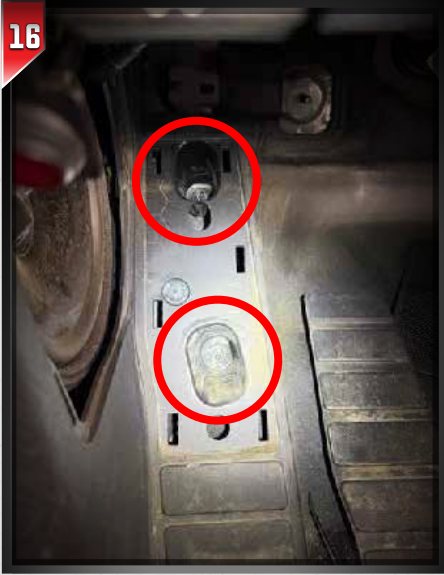
Now remove the drivers side panel along the footwell. It is held in with two screws and clips holding it into place. You will need to remove a small panel mounted to it to expose the 2, 10mm bolts. Once you have removed those you can fully remove the entire panel.
