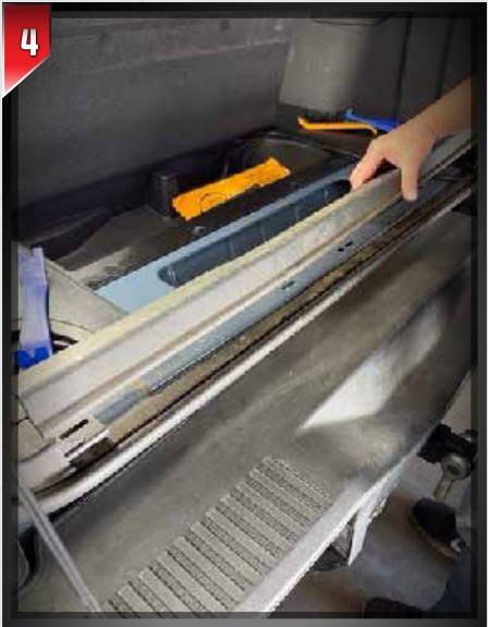
4 Remove the tail gate panel using a panel popper.
