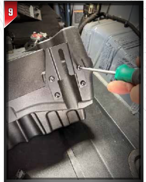
9 Install the 3 brackets to the sub box, using a T30 torx wrench and provided hardware.
