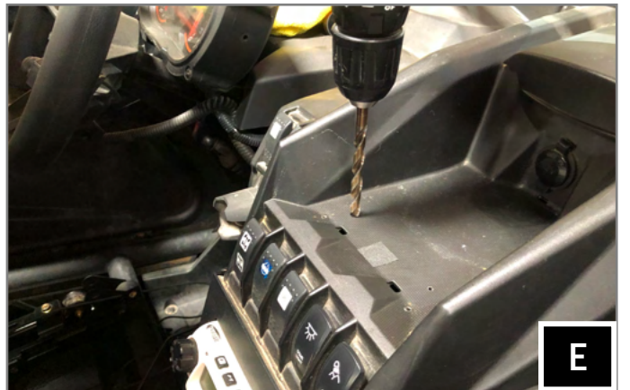
E. Cut out the traced circle. Limit speed and depth of cutting device to avoid damaging any wiring.
