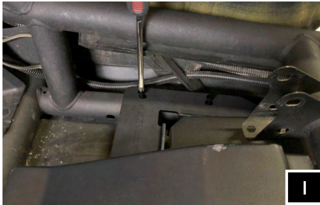
I. The large bracket will align over (2) factory holes in the chassis. Using a #3 Phillips screwdriver, secure the large bracket to the chassis with the provided (2) thread rolling screws and washers.
