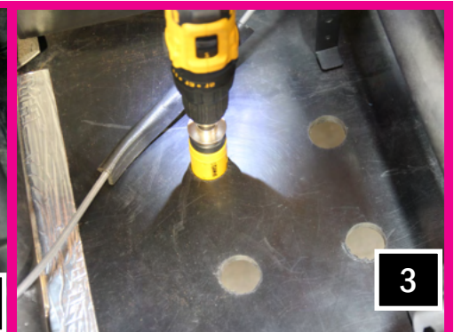
H. To help minimize skid plate rattle, we have supplied a drill template that adds 4 holes to help relieve air pressure that is being generated by the high output of the sub enclosure. Use the mounting bracket for the front of the sub enclosure for reference. Line up the template under the sub mounting brackets. (1). With hole punch/scribe tool mark the 4 drilling points through the template on to the floorboard (2). Drill the four (4) - 1 1/2" holes with a hole saw (3).
