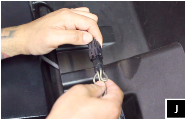
J. Plug the open end of the B-H3081 "Y" harness to the X32-PUS10 (passenger side).
