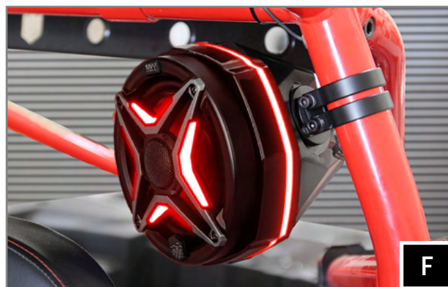
F. Route the rear speaker "Y" harness away from any moving parts and any sharp metal, then connect to the cage pods.
