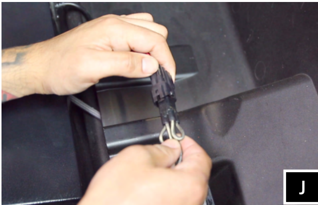
J. Route the B-H2702 sub extension harness along the center console away from any moving parts and sharp metal towards the rear of the vehicle then connect to the B-H3081 "Y" splitter. Plug one end of the "Y" splitter to the B-H3074 2-pin extension (3 ft) to the X32-DUS10 (driver side).
