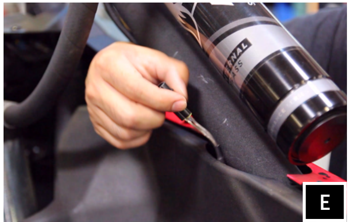
E. Route the rear speaker harness along the factory wires in the engine compartment and pull up through the small space between the bed panel and cage tubing on both passenger and driver sides.
