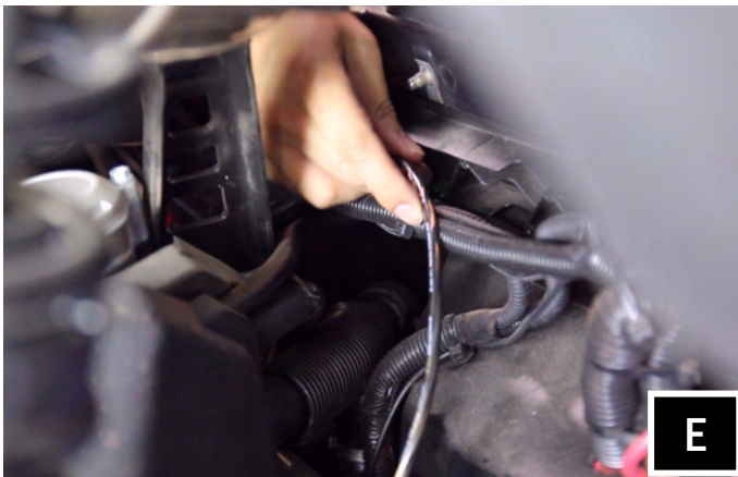
E. Route the rear speaker harness along the factory wires in the engine compartment and pull up through the small space between the bed panel and cage tubing on both passenger and driver sides.
