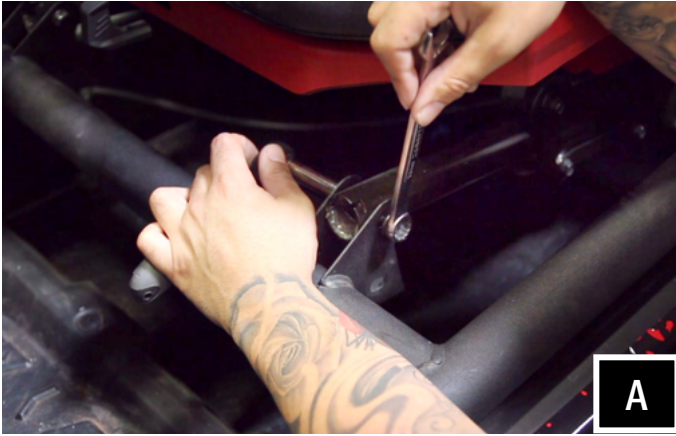
A. To remove the seat, use a 13mm socket and wrench to remove front (2) bolt and nut, and use a 18mm socket to remove (2) rear nuts and seat belt nut (repeat on other seat)
