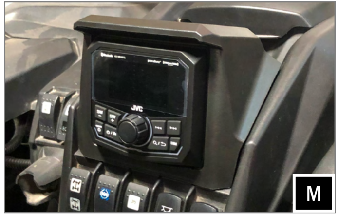
M. Center the trim ring on the MR1 and firmly press down until the side and corners click into place.
