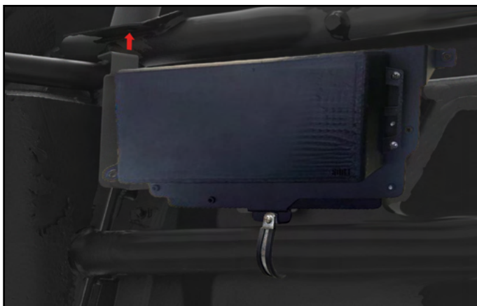
The amp tray mounts on the driver side firewall above the tube chassis.
