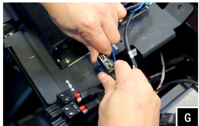
G. Connect the B-H1913 & B-H1912 speaker harness to the amplifier 800.5 rear output.
