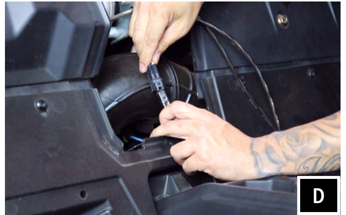
D. Take the B-H2195 rear speaker harness and plug into the B-H1913 & B-H1912 rear extension harness.
