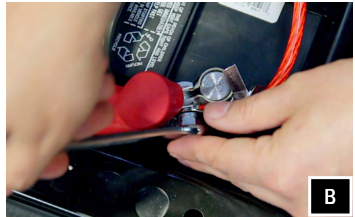
B. Unscrew the factory nut on the positive battery terminal. Install the 2 power cables to the screw on the positive battery terminal. Re-install the factory nut.
