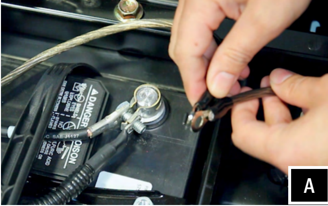
A. Unscrew the factory nut on the negative battery terminal. Install the 2 ground cables to the screw on the ground battery terminal. Re-install the factory nut.
