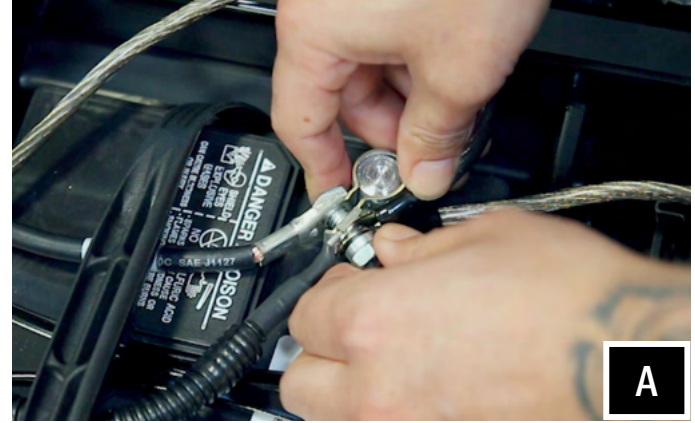
A. Unscrew the factory nut on the negative battery terminal. Install the 2 ground cables to the screw on the ground battery terminal. Re-install the factory nut.
