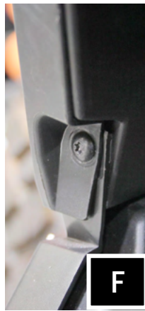
F. Remove fender well panel using a T30 driver (will need a 10mm socket for the screw near the headlight)
