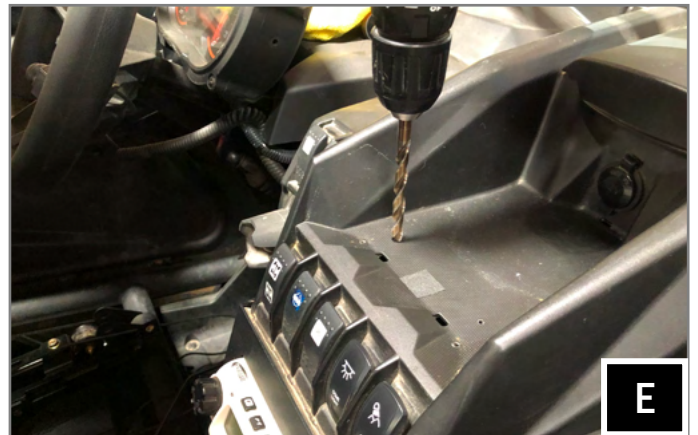
E. Cut out the traced circle. Limit speed and depth of cutting device to avoid damaging any wiring.
