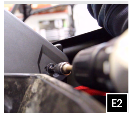
E2. Using panel removal tool unsnap (2) push clips on the driver and passenger side dash covers. Unscrew the (4) T30 screws on the passenger side, and (7) T30 screws on the driver side.
