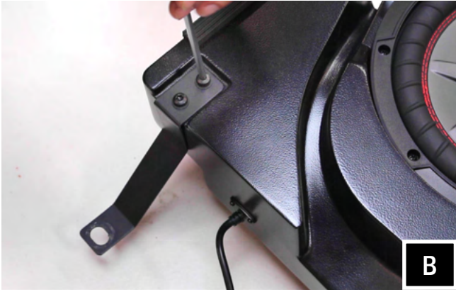
B. Using the supplied T-30 torx M6 screws and washers, screw the C bracket to the bottom left side of the enclosure.
