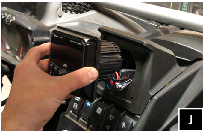
J. Place the MR1 into the DMR1. When placing the MR1 into the dash mount, feed slack wiring back into the dash cavity cut out. This will allow for proper fitment of the MR1.
