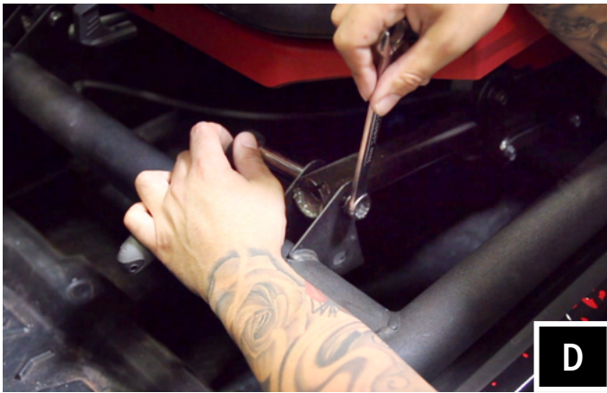
D. To remove driver the seat, use a 13mm socket and wrench to remove front (2) bolt and nut, and use a 18mm socket to remove (2) rear nuts and (1) 16mm seat belt bolt. Disconnect the seat belt sensor.
