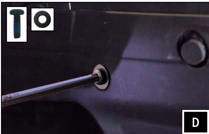
D. From the outside of the firewall, use the included M6 x 16mm screw and washer to secure the amp plate through the hole you drilled on the firewall.
