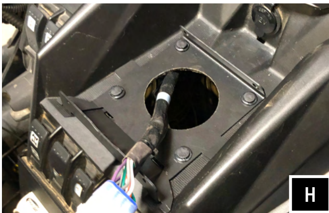
H. Route the MR1 power harness and 500.1 audio input and any other related accessories out of the cutout.
